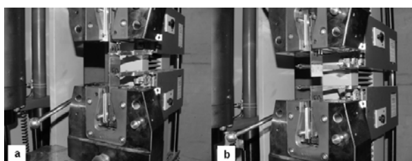
Fig. 8.1: Tension-shear test of single overlap joints before and after failure.
