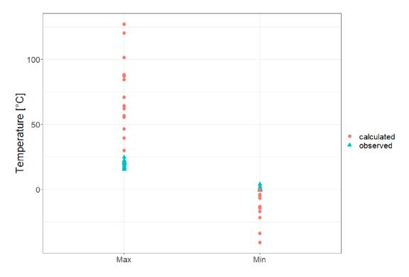
**FIGURE B2** Comparison of calculated and observed minimum and maximum values for all waterbodies. Calculated values were determined by MinMax analysis, observed values were retrieved from the datasets.
