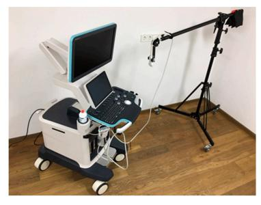
Figure 6. Ultrasound probe with fixation arm.
