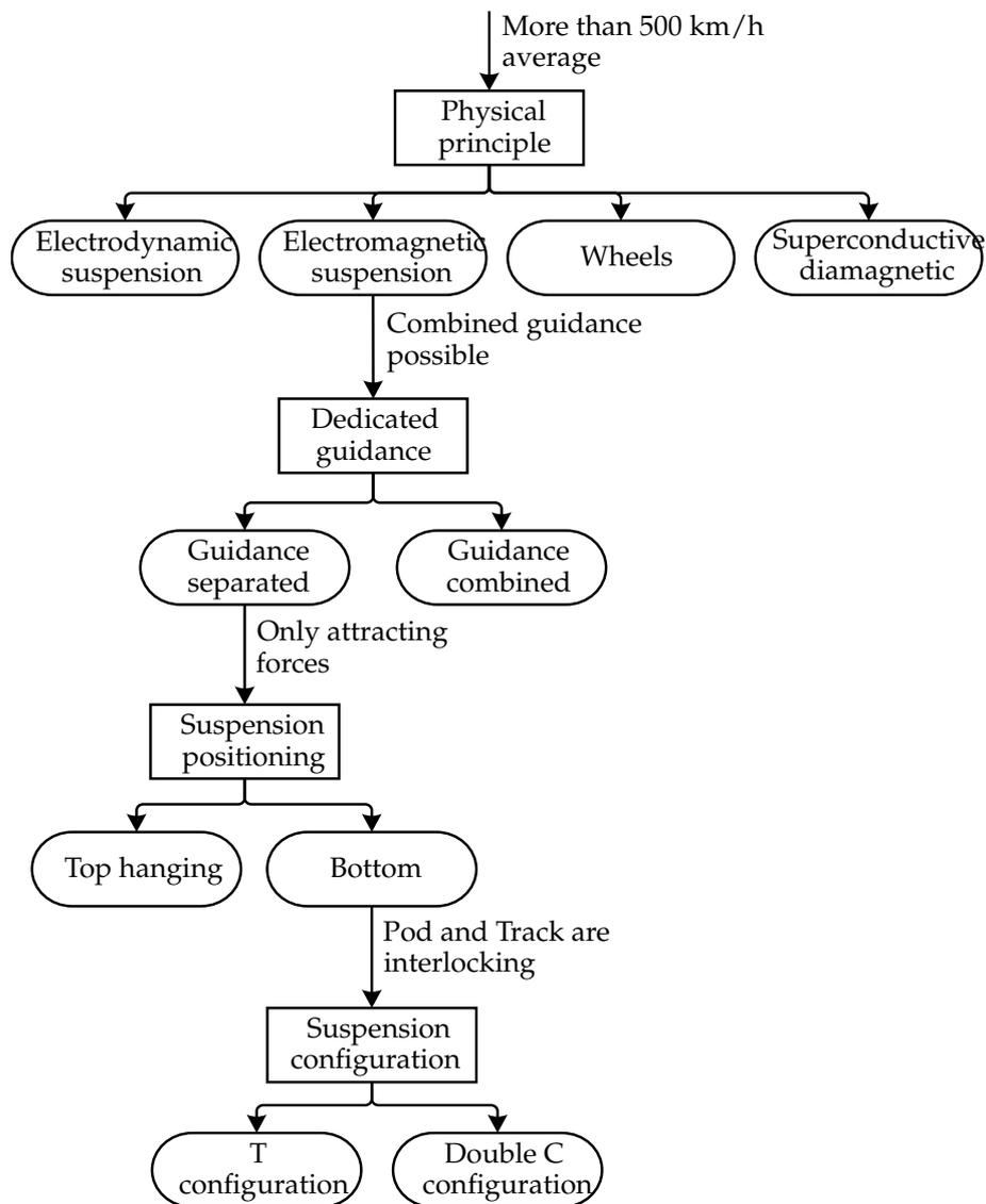
**Figure 3.** Design decision tree for the suspension system addressing the physical suspension principle; whether or not to separate the guidance, the positioning and the configuration.
