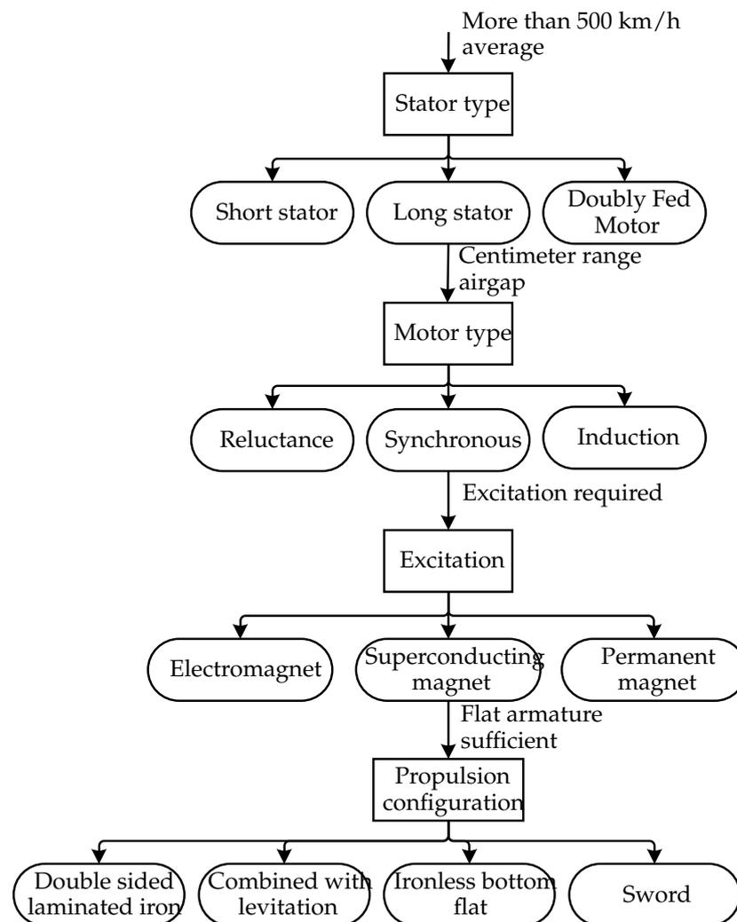
Figure 4. Design decision tree for the propulsion system.
