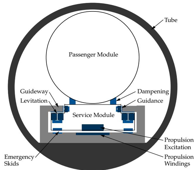
**Figure 5.** Schematic of the derived TUM Hyperloop Concept proposal. Electrically powered components are colored dark blue. Passive components are light blue or gray.
