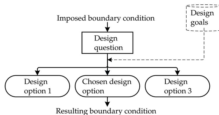
**Figure 2.** Template for the visualization of the DDT framework. Design decisions are presented as a design question followed by the available design options and based on the imposed boundary conditions and design goals.
