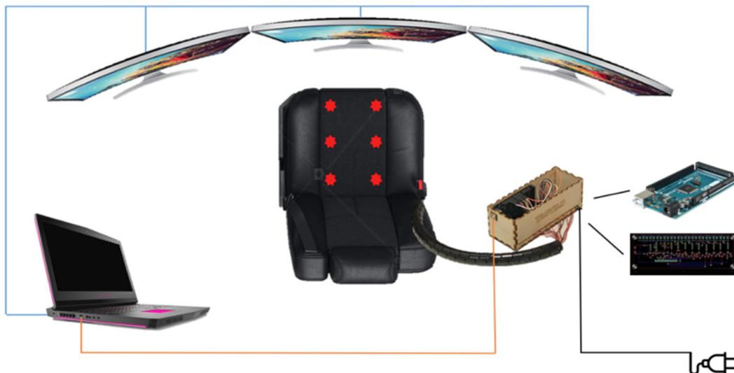
**Figure 4.** Hardware setup of the driving simulator consisting of three simulation monitors (**top**), the driver's seat with the advanced driver assistance system (ADAS) embedded in the seat cover as viewed from above (**central**), the simulation computers (**left**) and the ADAS control unit consisting of a microcontroller, Printed Circuit Board (PCB), and wiring (**right**).
