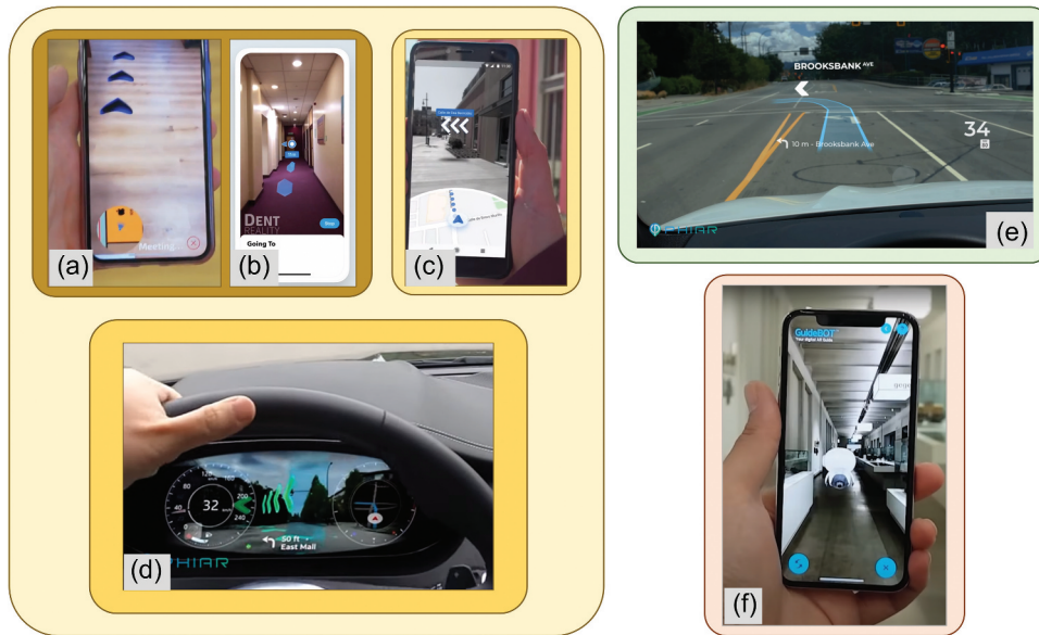
Figure 2. Typical visualization styles of direction. (a)-(d) separate arrows/dots, (e) separate arrows with consecutive lines, (f) animated avatar.
