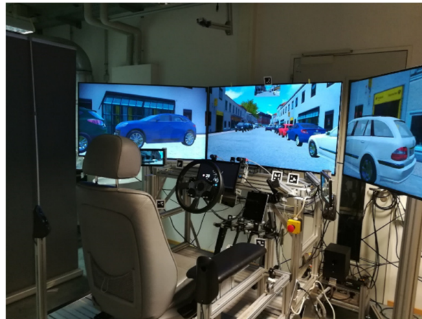
Figure 4. Mock-up with three 55" ultra-HD monitors creating a 120° field of view, 13" monitor for the IC, and tablet.
