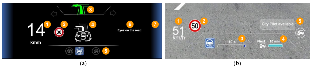
Figure 1. (a) IC with current speed (1), speed limit (2), navigation (3), maneuver (4), automation scale (5), L2-specific driver task (6), and level of automation color in the frame (7); (b) HUD with current speed (1), speed limit (2), predictive element for current (3) and upcoming segment (4), and availability pop-up message for City Pilot (5).
