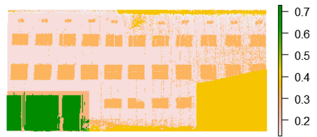
Fig. 7. Probability texture: BayNet estimates the probability for each pixel for the target node state underpass .
