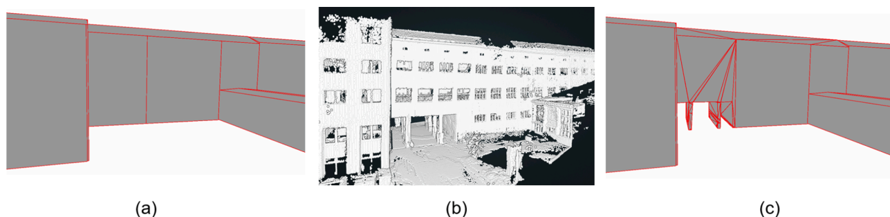
Fig. 12. Semantic 3D building model refined by the addition of an underpass using MLS point clouds. a) Raw city model, b) point cloud, c) refined building model.
