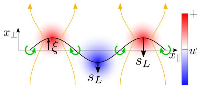
**Figure 6.** Flame-generated vorticity at a corrugated flame sheet—indicated by green circular arrows—increases and decreases flow speed, as indicated by the red and blue areas as well as the orange stream tubes. Variations of flame speed as a result of flame stretch are indicated by downward pointing small arrows of various lengths.
