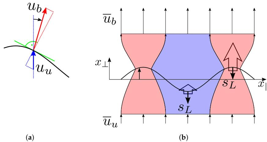
**Figure 12.** (a): Downstream of a flame, velocity vectors are bent towards the flame normal direction, since the flow accelerates across the flame front. (b): The instability of a flat flame sheet results from contraction (red) and expansion (blue) of flow tubes across a corrugated flame front that can be linked to consequences of flame generated vorticity (captured by the BD model) and irrotational contributions of flow expansion (not captured).
