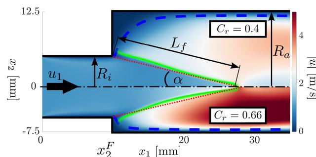
**Figure 7.** CFD steady state absolute velocity for a confinement ratio of  $C_r = 0.4$  (upper half) and  $C_r = 0.66$  (bottom half). For both configurations, the location of maximum heat release (—), the analytically predicted mean flame front (· · · · ·) and the approximate location of the shear layer (---) are also shown.
