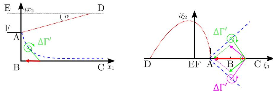
**Figure 3.** Illustration of how impermeability boundary conditions are met by use of a mirror vortex (not to scale): the wall normal velocity component of the original vortex of strength  $\Delta\Gamma'$  (green) is canceled by its mirror counterpart (pink) such that the resulting velocity (red) is parallel to the walls in the physical (left) as well as in the image domain (right). The shear layer and the flame front are shown as blue dashed and red dotted lines, respectively.
