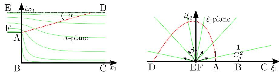
**Figure 2.** Illustration of the Schwarz–Christoffel mapping (not to scale). Mean flame position (.....) and straight lines radiating from the origin of the image domain (—), each in the physical domain (left) and the image domain (right).
