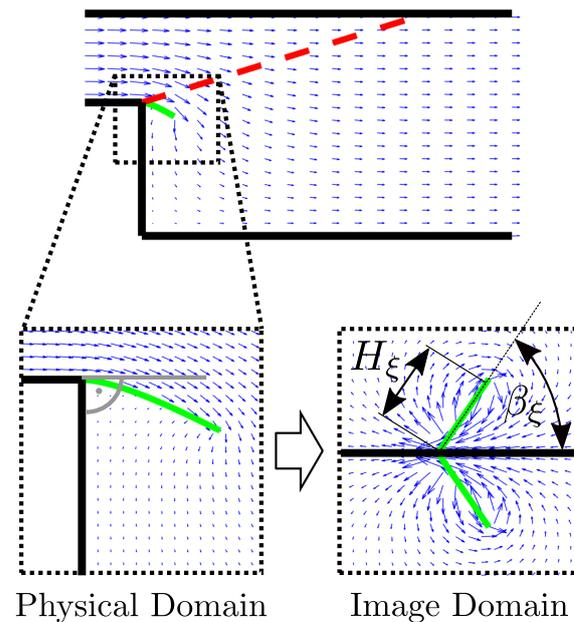
**Figure 4.** Flow field in a combustor with  $C_r = 0.4$  resulting from a source at  $\xi = 0$  and a Kutta panel (green). Close up views of the Kutta panel  $H_\xi = 2.1$  and  $\beta_\xi = \pi/3$  are shown in the physical (bottom left) and the image domain (bottom right).
