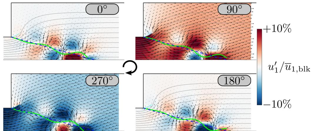
**Figure 13.** Predictions obtained with the BD model of a flame with confinement ratio  $C_r = 0.4$  forced harmonically at 120 Hz and an amplitude of  $10\% \bar{u}_{1,blk}$ . Color raster: axial velocity  $u'_1$ ; mean flame front (---); perturbed flame (—). Minimum vortex kernel radius  $r_{0,\omega,min} = 4.25 l_M$ .
