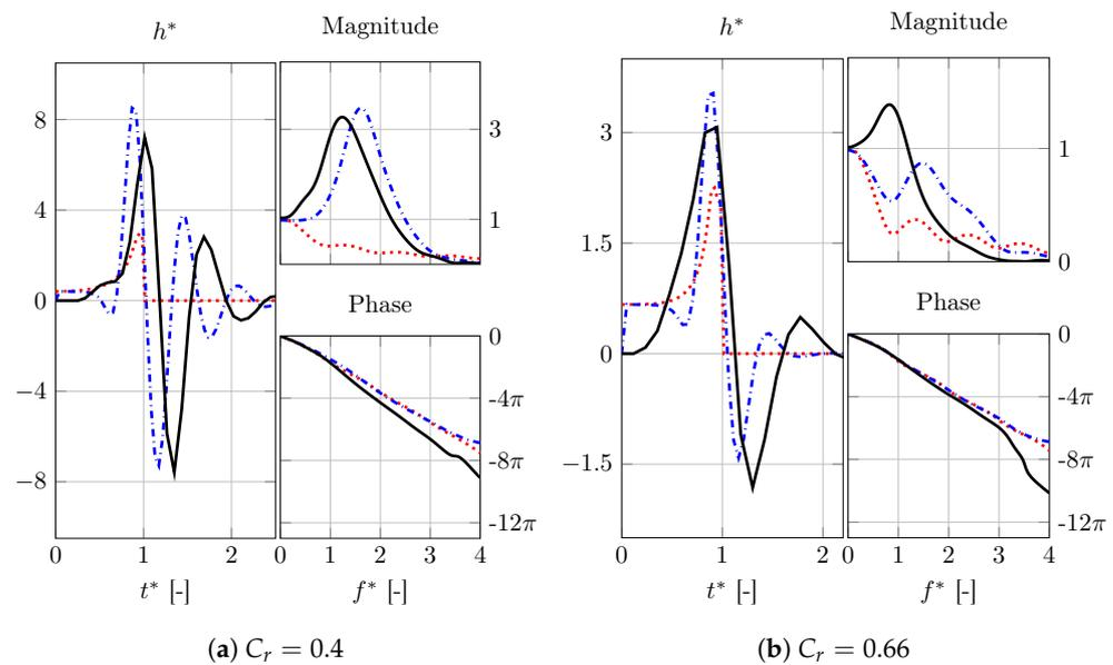
**Figure 11.** Impulse responses (left plot in sub-figures (a,b)) and frequency responses (right plots in sub-figures (a,b)). CFD results (—) vs. predictions of the unidirectional (•••••) and bidirectional (---) models, that is without and with consideration of flame-generated vorticity ( $r_{0,\omega,\min} = 4.25l_M$ ).
