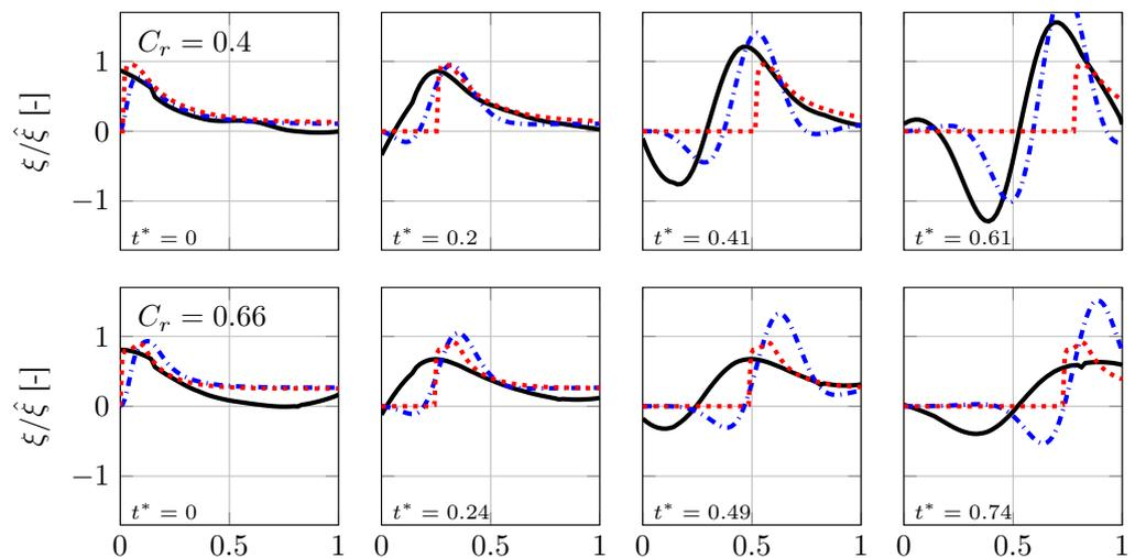
**Figure 10.** Four snapshots taken at equidistant instances in time of the normalized flame displacement plotted over  $x_{||}/L_f$  resulting from an impulsive velocity forcing at  $t^* = 0$  for confinement ratios  $C_r = 0.4$  (top) and  $C_r = 0.66$  (bottom). CFD results (—); UD model (····); BD model (-·-·-).
