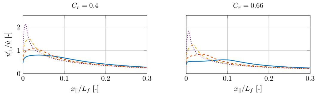
**Figure 9.** Flame normal velocity perturbation along the flame length resulting from Kutta conditions with panel lengths  $H_{\zeta}$  (—),  $H_{\zeta}/2$  (---),  $H_{\zeta}/4$  (····) and  $H_{\zeta}/8$  (-·-·-).  $H_{\zeta}$  is set to 2.1 for  $C_r = 0.4$  (c.f. Figure 4) and to 1.8 for  $C_r = 0.66$ , respectively.
