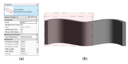
**Figure 13.** Visualization of dimensional disconformity—machine system's workspace is smaller than the dimension of a single curved wall. (a) A parametric Revit family represents the workspace and is controlled by the BIM toolkit. (b) The workspace is automatically positioned and oriented on the curved wall.
