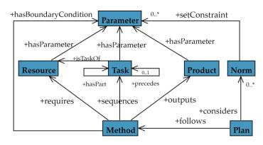
**Figure 5.** Conceptualization principle: planning incorporating the PPR model. Unless specified, the cardinality of the associations is set to "1..\*".
