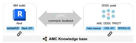
Figure 11. Technical framework for the knowledge-driven DDSS (redrawn from [42]).
