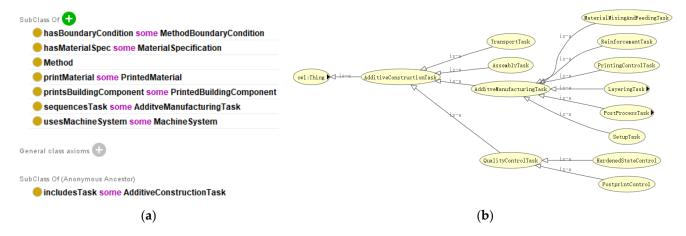
**Figure 8.** (a) Important entities related to AM methods; (b) Taxonomy of tasks defined by additive manufacturing plan.
