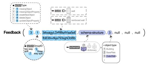
Figure 14. Feedback function for structural rework (redrawn from [48]).
