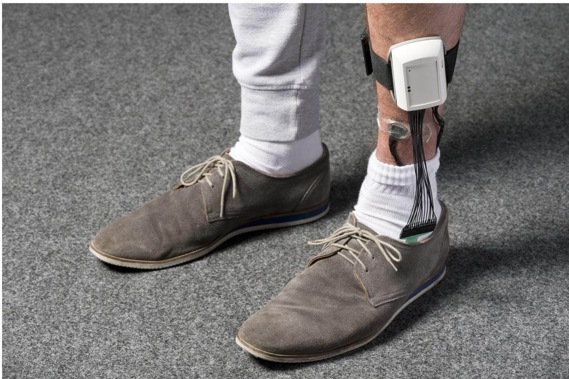
**Figure 13.** Adapted KIPRODE sensor system to investigate the pressure load of risk patients at their feet during their daily life. The white box contains all electronics, whereas the small sensor node measures vital signs. The pressure sensor foils is inserted in the shoe (©Fraunhofer EMF/Bernd Mueller).
