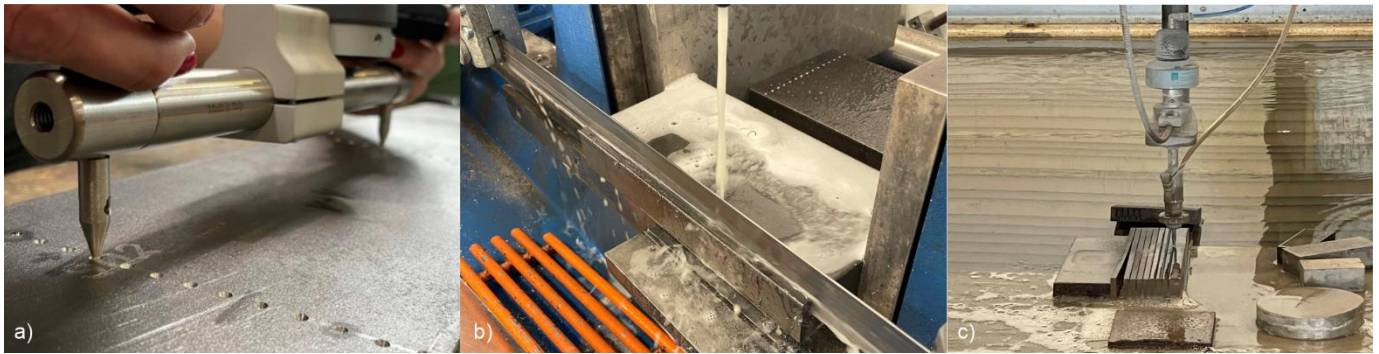
Figure 6 Steps of the sectioning method a) measuring initial distances, b) band sawing c) water jet cutting the segments.
