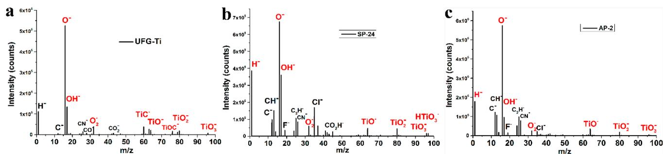
**Figure 3.** TOF-SIMS spectra of negative ions: (a) UFG-Ti; (b) UFG-SP-24; (c) UFG-AP-2.
