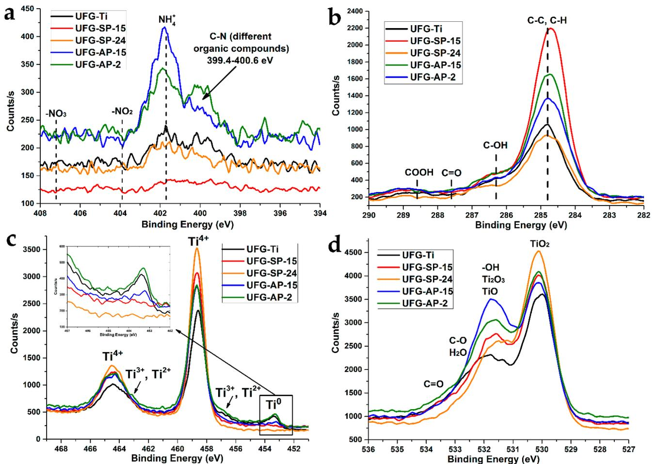
Figure 2. XPS spectra of polished and chemically etched UFG titanium: (a) N1s; (b) C1s; (c) Ti2p; (d) O1s.
