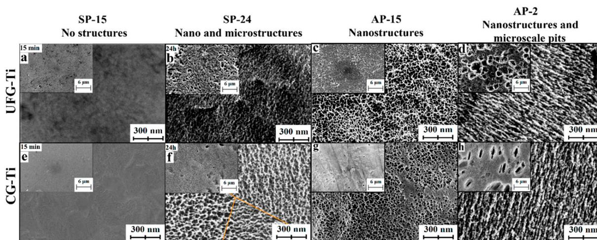
**Figure 1.** SEM images of chemically etched UFG and CG titanium discs: (a) UFG-SP-15; (b) UFG-SP-24; (c) UFG-AP-15; (d) UFG-AP-2; (e) CG-SP-15; (f) CG-SP-24; (g) CG-AP-15; (h) CG-AP-2. Reprinted with adaptation from [19].
