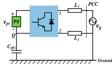
Figure 1. Typical single-phase grid-connected PV converter.
