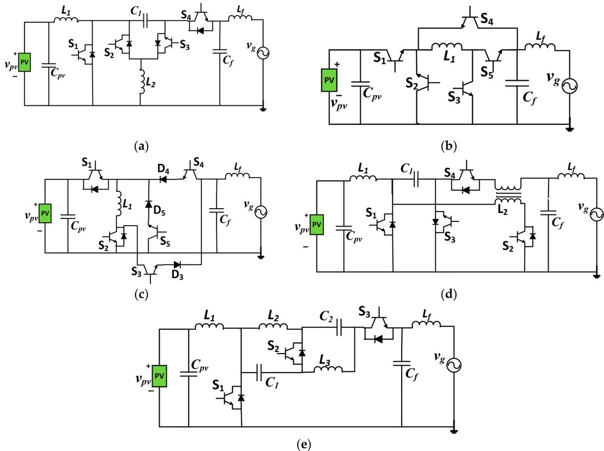
**Figure 3.** Current-source common-grounded (CSCG) converters. (a) Converter presented in the work of [36,37], (b) converter presented in the work of [38], (c) converter presented in the work of [39], (d) converter presented in the work of [40], (e) converter presented in the work of [41].
