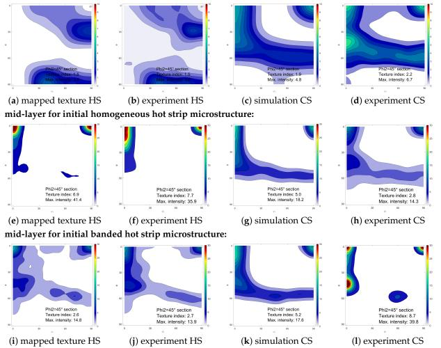
**Figure 7.** Comparison of experimental and simulation results for the texture evolution in Fe3.2wt.%Si steel. (**a**–**d**) Measured and predicted texture evolution near the surface of a homogeneous hot strip microstructure, (**e**–**h**) Measured and predicted texture evolution in the mid-layer of a homogeneous hot strip microstructure, (**i**–**l**) Measured and predicted texture evolution in the mid-layer of hot strip with a banded microstructure. HS—hot strip, CS—cold strip.
