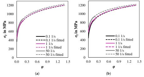
**Figure 5.** Experimental and extrapolated flow curves at room temperature determined by layer compression tests for hot strips with (**a**) a homogeneous microstructure and (**b**) a banded microstructure.
