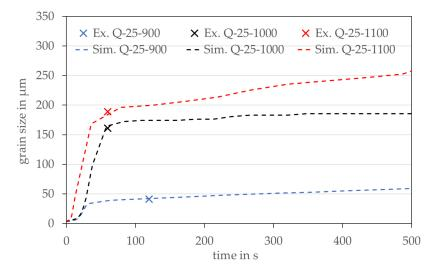
**Figure 10.** Simulated recrystallization and grain growth kinetics (dashed lines) based on grain size (y-axis) and time (x-axis) compared to individual experimental results (crosses). Data for experimental results are taken from [38].
