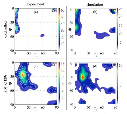
**Figure 12.** ODF  $\varphi_2 = 45^\circ$  section of the experimental (**a**) and simulation (**b**) cold rolling texture as well as the resulting experimental (**c**) and simulated (**d**) texture after annealing for 120 s at 900 °C.
