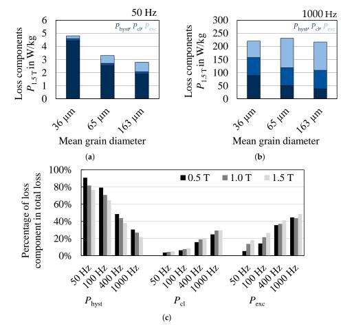
**Figure 20.** Loss component distribution at 1.5 T for three 0.25 mm thick non-oriented electrical steel grades at (**a**) 50 Hz and (**b**) 1000 Hz, and (**c**) loss component distribution for the sample with a mean grain size of 65  $\mu$ m and thickness of 0.25 mm.
