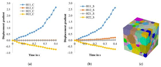
**Figure 6.** Displacement gradient in cold rolling of Fe3.2wt.%Si with a homogenous microstructure, (**a**) in the mid-layer and (**b**) near the surface. (**c**) Corresponding RVE with 300 grains used in both cases. 11—displacement gradient in normal direction, 22—displacement gradient in rolling direction, 12 and 21—displacement gradient indicating shear, C—mid-layer, S—near surface layer
