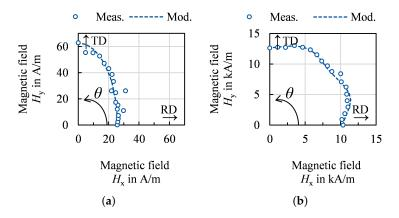
**Figure 18.** Comparison of continuously modeled and in 5°-steps measured magnetic field in the RD-TD plane at two different polarizations for a commercial M235-35A steel at 50 Hz, (**a**) at 0.3 T, (**b**) at 1.8 T.
