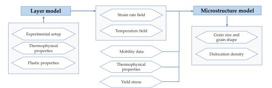
Figure 1. General input and output parameter for hot rolling model.
