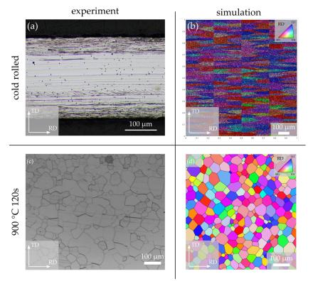
**Figure 11.** Light microscopy images of (**a**) the cold rolled and (**b**) the sheet annealed at 900 °C in comparison to the simulated microstructures (**c**) using the microstructure generator to produce the equivalent to the cold-rolled state and (**d**) the resulting microstructure after simulation of RX and GG.
