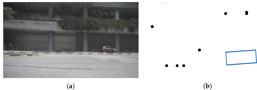
Figure 12. Vehicle in line-of-sight direction from the radar sensor. Despite its exposed position, it is not detected with the sensor settings used. (a) The vehicle in camera view in front of the sensor vehicle. (b) BEV: Zoom onto the GT bounding box in blue and the radar data in the surroundings. No radar return originates from the vehicle. NuScenes sample token: bbba31d91e334f4abf6d1f96bf699980.
