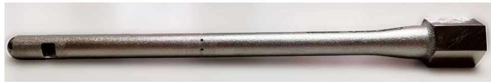
Figure 8. Additive manufactured probe after printing and the side opening to the axial heater cavity.
