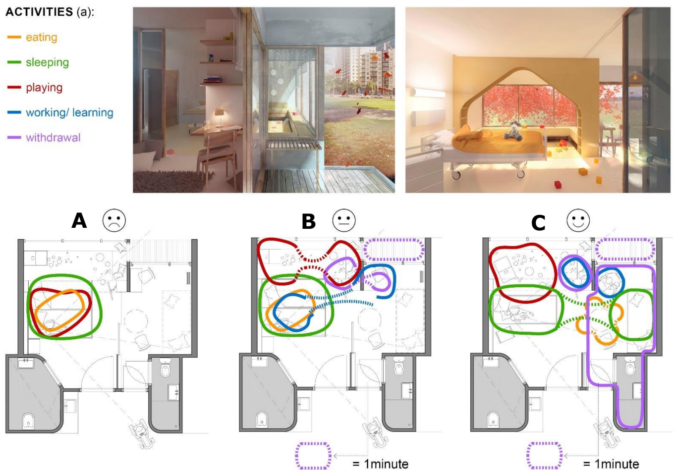
Figure 7. Graphical depiction of how the PCPU reacts to the association of parental distress and the three architectural determinants: (A) distance between parent and child; (B) used space for interaction; (C) used possibilities for withdrawal.
