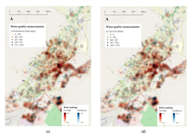
**Figure 5.** (a) Visual representation of the current risk of wastewater seepage into the groundwater of Leh Town. (b) Overlay of nitrate measurements [39]. (c) Overlay of TDS measurements [39]. (d) Overlay of *E. coli* measurements [39]. Water quality data reprinted with permission from ref. [39]. Copyright 2017, Christoph Schwaller.
