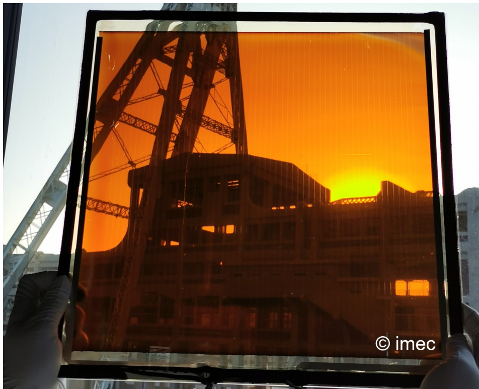
Figure 2.10: Bifacial semitransparent large-scale perovskite module by Imec [142]. Photograph from Imec unveils 781 cm 2 bifacial perovskite solar panel with 11.9% efficiency (pv-magazine.com), accessed 12.07.2023.
