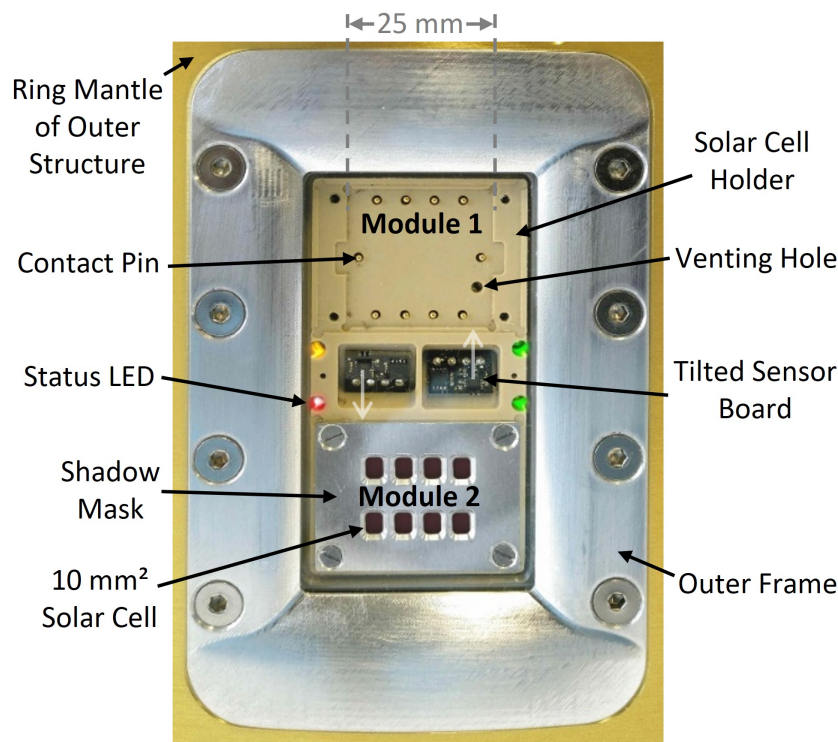
Figure 4.5: Outside close-up view of one of the eight hatches with the plugged-in insertion module. Behind the fused silica window (barely visible), the beige solar cell holder for two solar cell modules is visible. At module position 1 the spring pins for solar cell contacting are visible, in position 2 the shadow mask is assembled, defining eight solar cells with each 10 \text{ mm}^2 aperture. Between the solar cell modules, two tilted sensor boards (one facing upwards, one facing downwards, indicated with the white arrows) are placed to collect illumination and temperature information. Reproduced from Reb et al. with permission [215], copyright 2021 the Authors.
