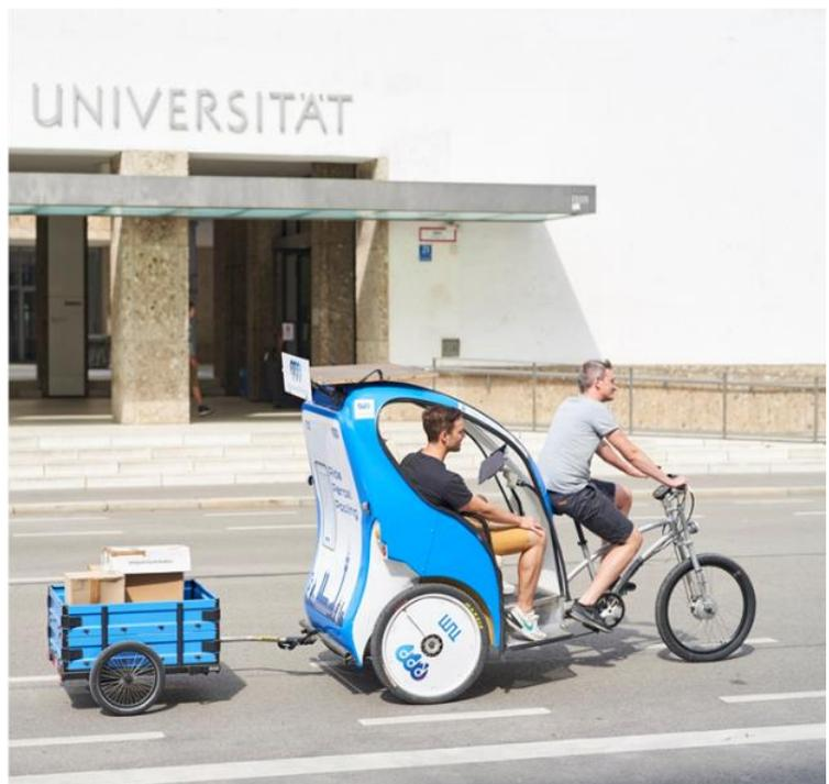
Figure 6 – RPP rickshaw (prototype for the integrated transportation of passengers and freight).
