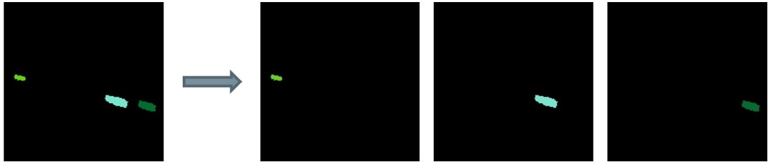
Figure 3.15: An illustration of extracting individual RGB color for the preparation of bounding box generation.
