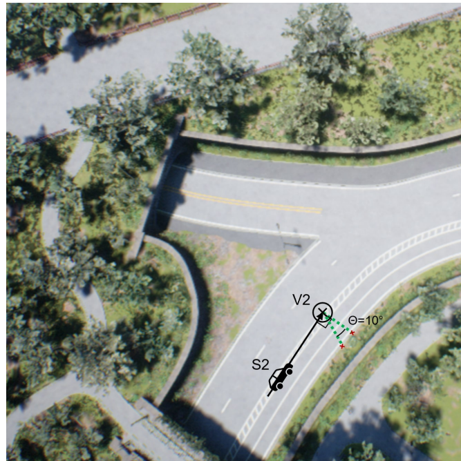
Figure 3.11: Step of finding the orientation at new location V2. Green dots indicates that the line trace encounters road; red crosses indicates the line trace doesn't encounter road.
