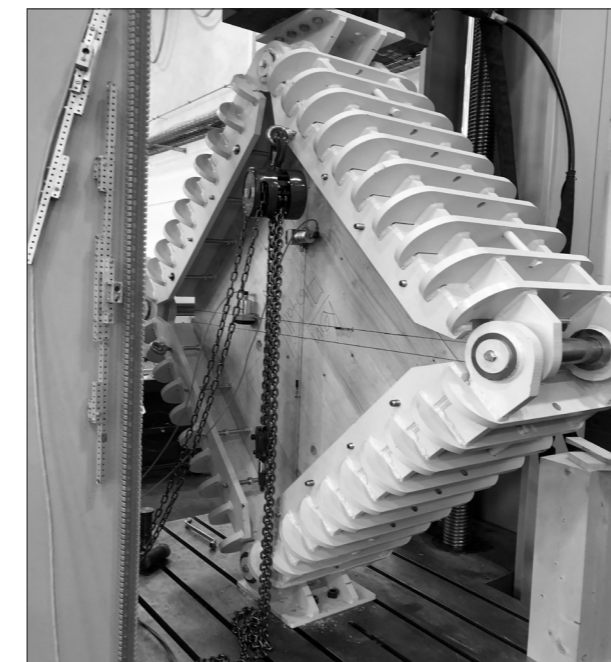
Fig. 2.4: Determination of the in-plane shear stiffness using shear frame tests
