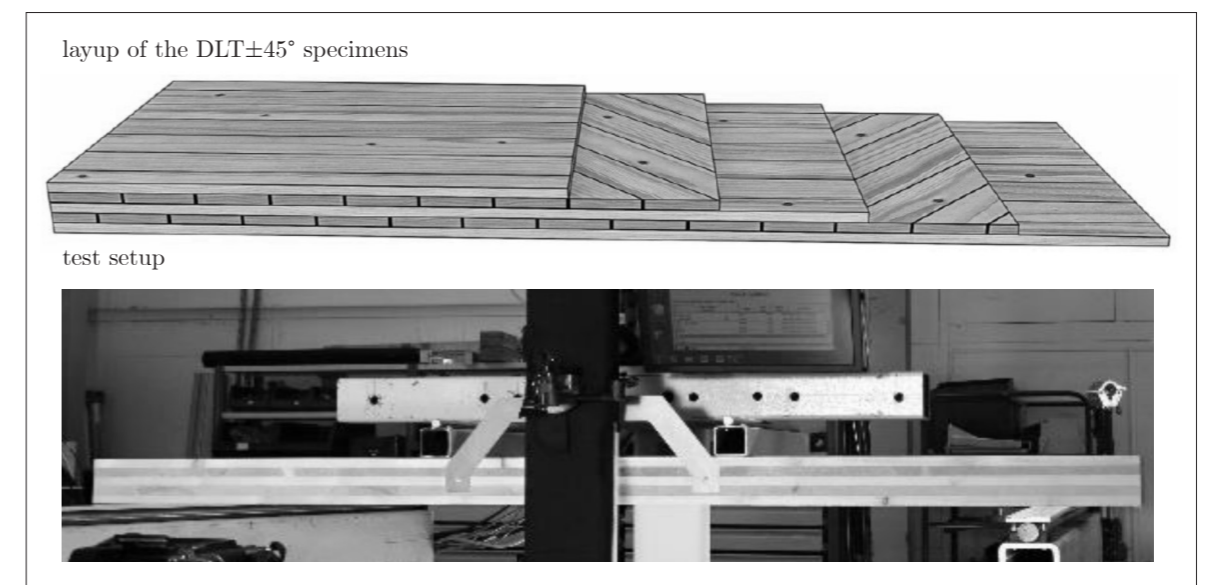
Fig. 1.10: DLT panel with alternating layer configuration in four-point-bending tests (BUCK ET AL 2016)
