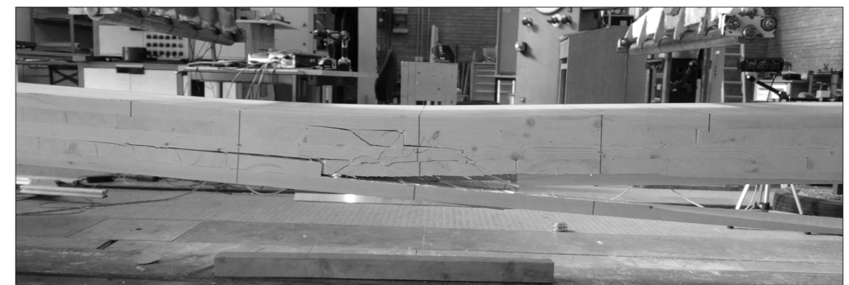
Fig. 7.6: Display of an exemplary failure mechanism in bending of D1-4 specimen
