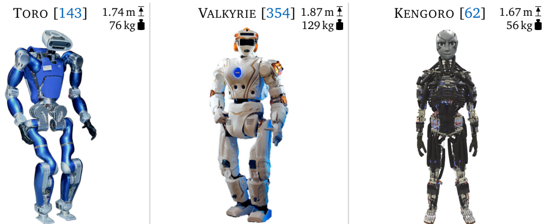
Figure 2.9: Full-sized humanoid robots following non-conventional design approaches. From left to right: TORO (based on LWR III robotic arms) by DLR, VALKYRIE (incorporates SEAs) by NASA, and KENGO (musculoskeletal humanoid) by the University of Tokyo . Images modified from [62, 137, 354].
