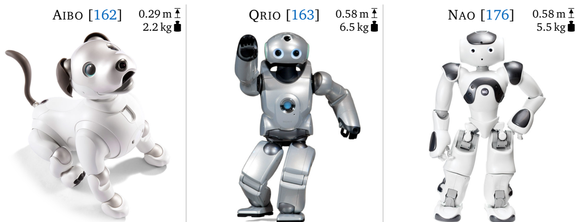
Figure 2.1: Small sized, commercial quadruped and humanoid robots. From left to right: toy robots AIBO and QRIO by Sony and research platform NAO by SoftBank / Aldebaran Robotics . Images modified from [383, 386, 387].
