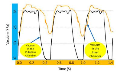
**Figure 1.** Cyclical vacuum fluctuations in the pulsation and inner chambers of the teat cup (Bio-Milker teat cup liners, Siliconform) during milking in the sheep milking machine with the following settings: vacuum level 38 kPa, pulsation rate 120 cycles/min and pulsation ratio 60:40 [7].
