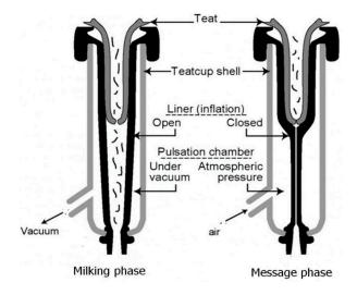
**Figure 2.** Suction phase (milking phase) and relief phase (massage phase) in mechanical milk removal according to Krömker [31] with some changes.
