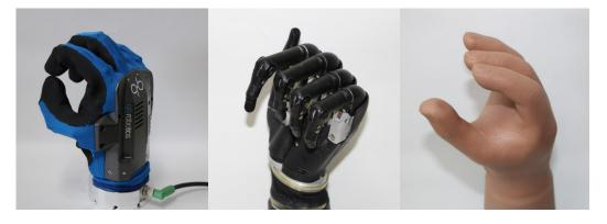
**Figure 2.** The different types of artificial hands used in the study: the qb SoftHand QBRobotics), the iLimb-Ultra (Ossur), and the VariPlus Speed (Ottobock).
