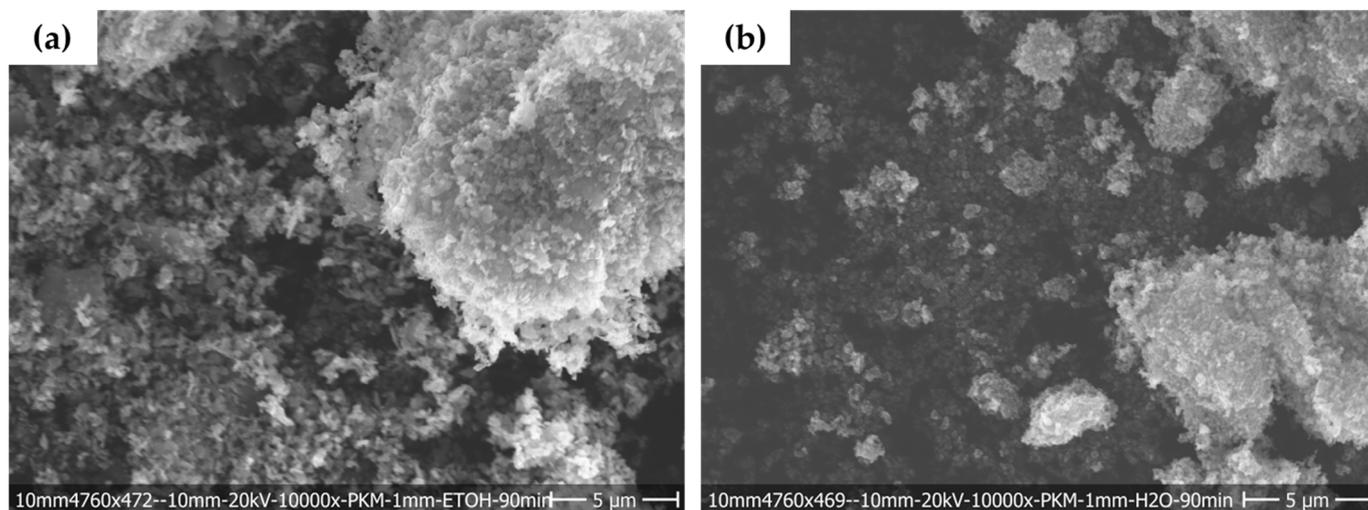
**Figure 1.** SEM picture of MNOs ground in the planetary ball mill while suspended in ethanol (a) and water (b). Pictures of the particles after a 90 min grinding process.
