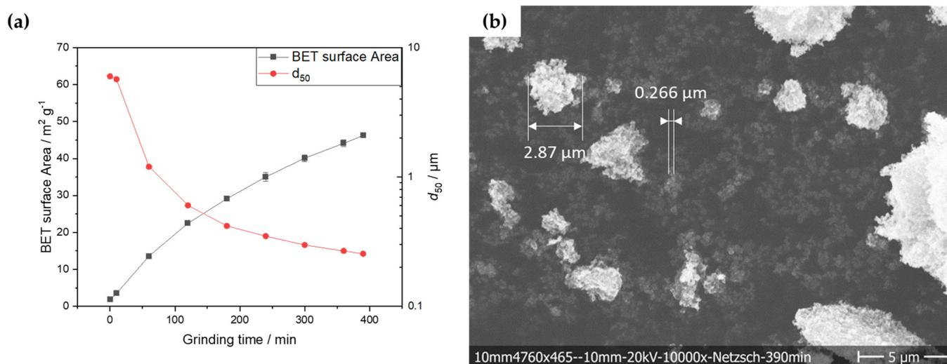
**Figure 5.** (a) Particle size and BET surface area during grinding of magnetite ore in an agitator bead mill (LabStar Zeta, Netzsch Feinmahltechnik GmbH); (b) SEM picture of MNOs produced after 390 min grinding in an agitator bead mill.
