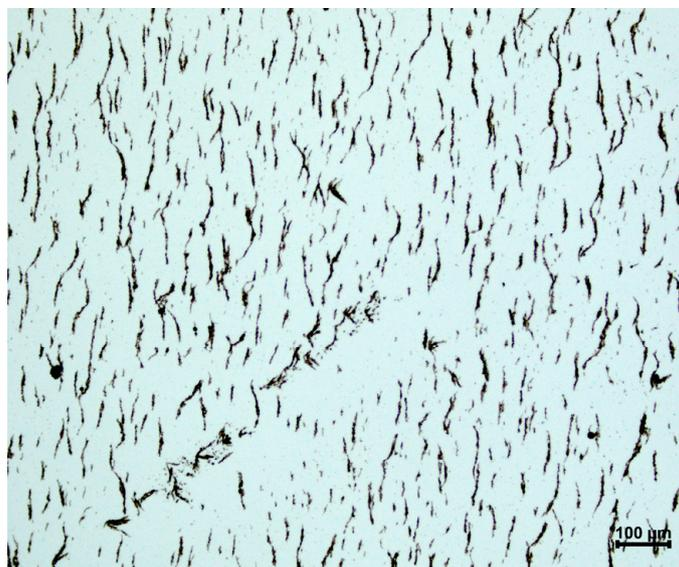
**Figure 2.** Brightfield image of magnetite ground in 75 mM sodium phosphate buffer for 90 min, 1 mm zirconia beads, 100× magnification.
