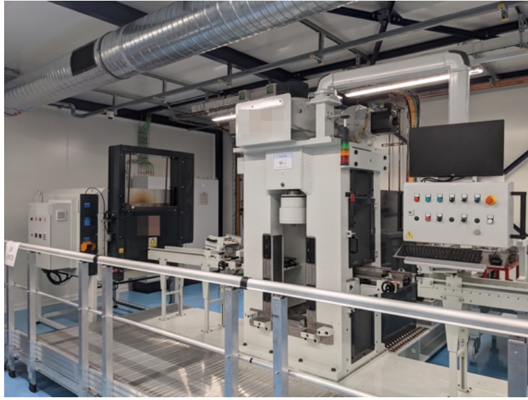
Figure 10.1: Hot-rolling machine implemented in CERCA TM laboratory
