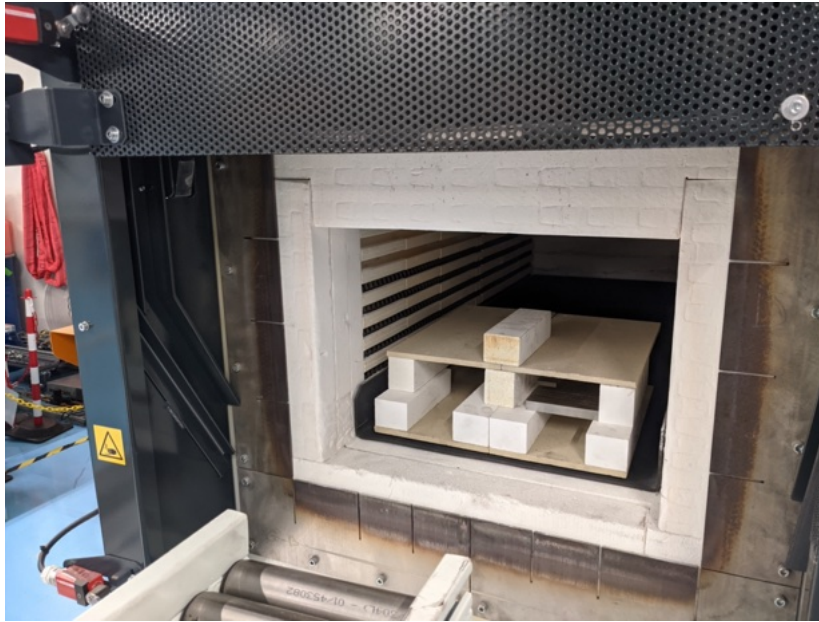
Figure 10.2: One ceramic support configuration used for sample holding during rolling process
