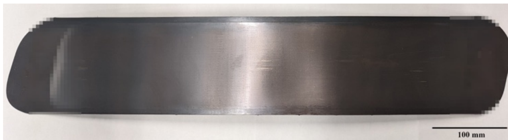
(a) Welded assembly overview after hot rolling process
