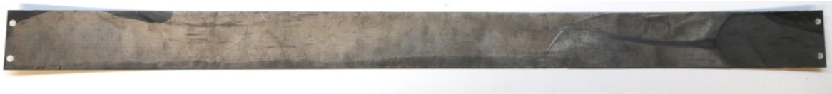
(b) Bottom surface of U-10Mo bare foil
