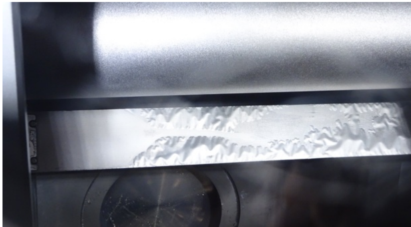
Figure 11.36: Non-sticking of zirconium on the U-10Mo bare foil with surface contamination
