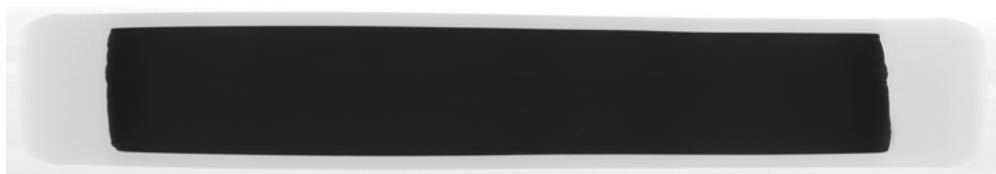
(b) RX-ray transmission pictures of U-10Mo foil (in black) in stainless steel canister (in grey)
