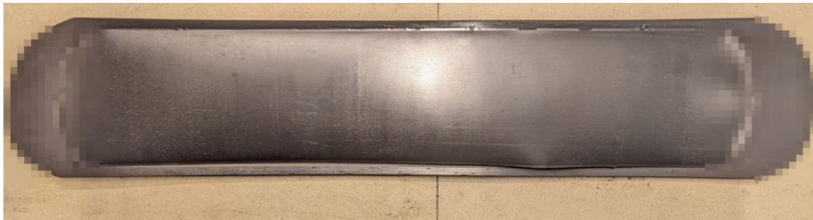
Figure 11.7: Welded stainless steel assembly after the rolling process with cracks
