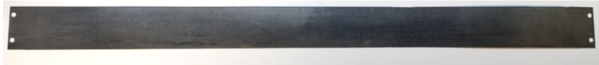
(a) Top surface of U-10Mo bare foil
