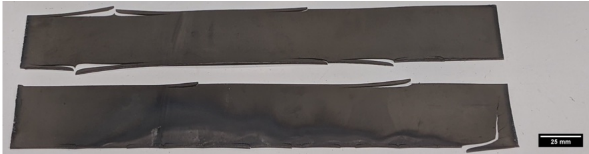
Figure 8.12: U-10Mo bare foil with edges cracks after laser cutting resizing
