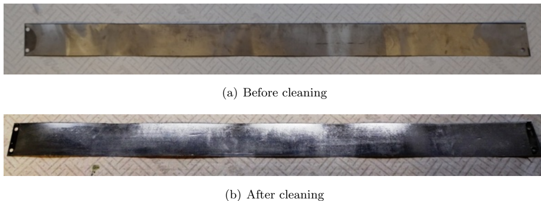
Figure 11.35: U-10Mo bare foils before and after electrochemical cleaning for PVD coating
