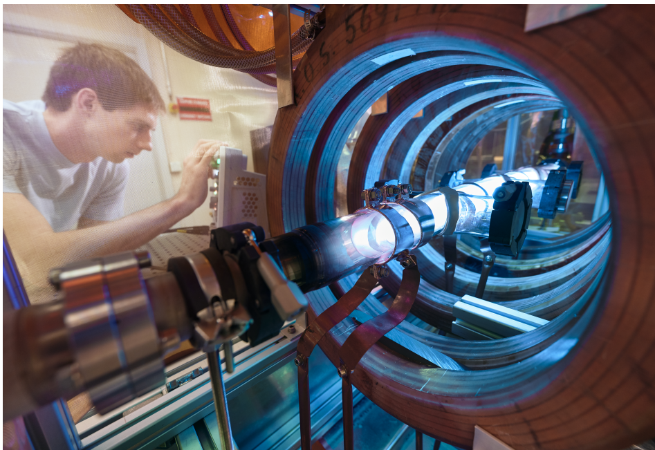
Figure 1.15: Helicon plasma cell in development for AWAKE. Image from [70].
