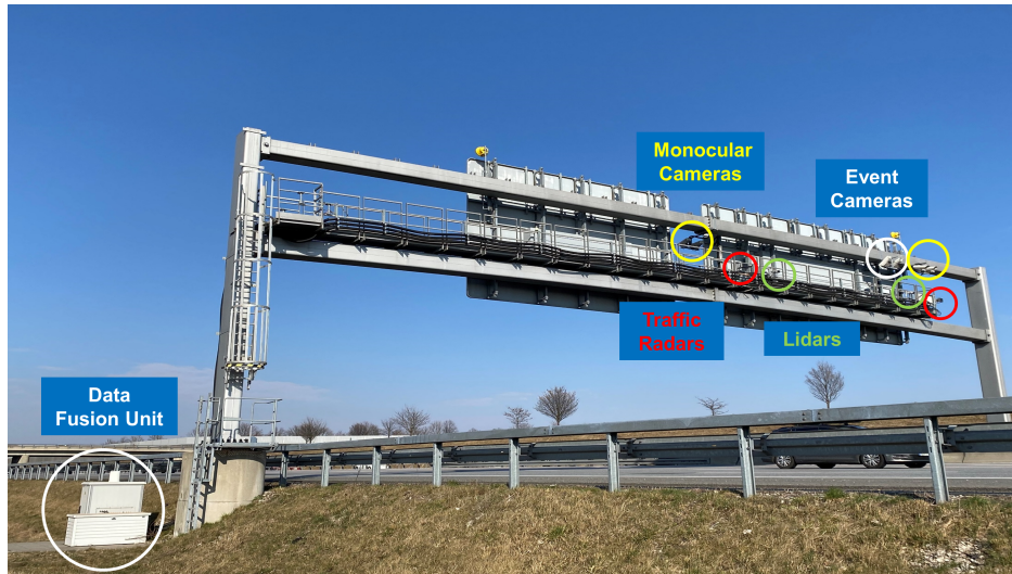
Figure 1.1: One of the measurement points on the highway A9 from Providentia++ project ( https://innovation-mobility.com/en/project-providentia/ ). Adapted from Fig. 1 in [Li+23d].
