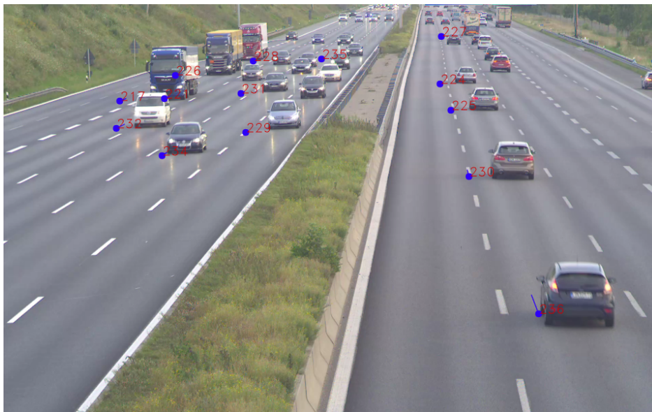
Figure 3.1: This is the image after the traffic radar measurements being projected onto the camera picture. The measurements (blue points) are sparse and contain biases and misdetections caused by noise.
