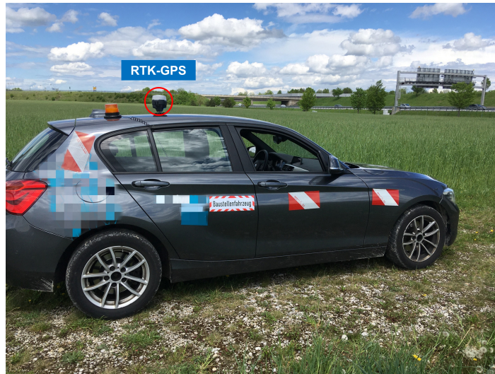
Figure 3.13: This is the test car with a high-precision RTK-GPS device (cm-level).
