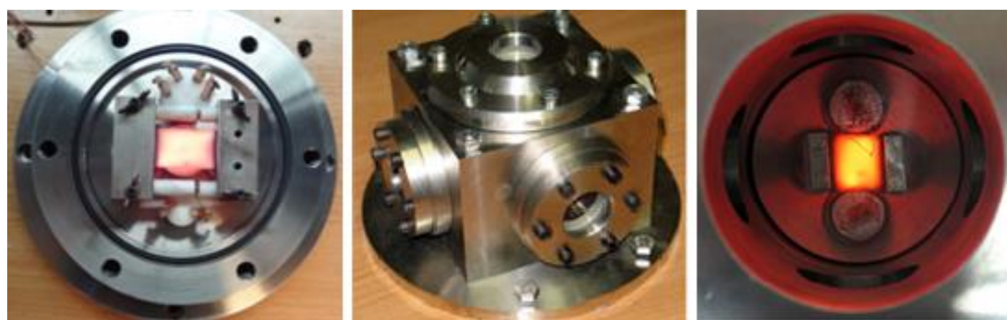
Fig. 1: Pressurized Wired-Mesh-Reactors (PWMR) provides kinetic devolatilization data for accurate entrained-flow gasification modelling and CFD studies.
