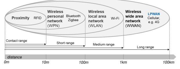
Figure 1 Types of wireless communication networks and their ranges (based on Ibrahim 2019)
