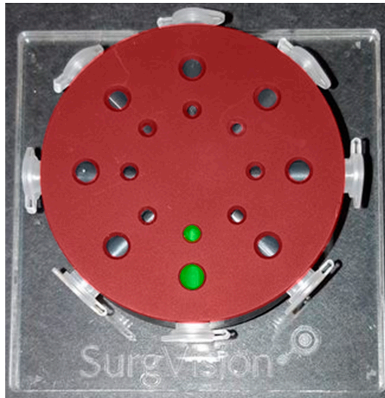
Figure A1. CalibrationDisk with regions of interest and background highlighted. The CalibrationDisk for near-infrared fluorescence calibration with eight transparent Eppendorf tubes. Regions of interest (ROIs), defined as the windows in the CalibrationDisk of one sample, are displayed in green. Background was defined as the surface of the CalibrationDisk around the ROIs, displayed in red. The caps of Eppendorf tubes could show fluorescence, however, this was not considered as visible or an ROI. ROIs and background were used to calculate target-to-background (TBR), signal-to-noise (SNR), and contrast-to-noise (CNR).
