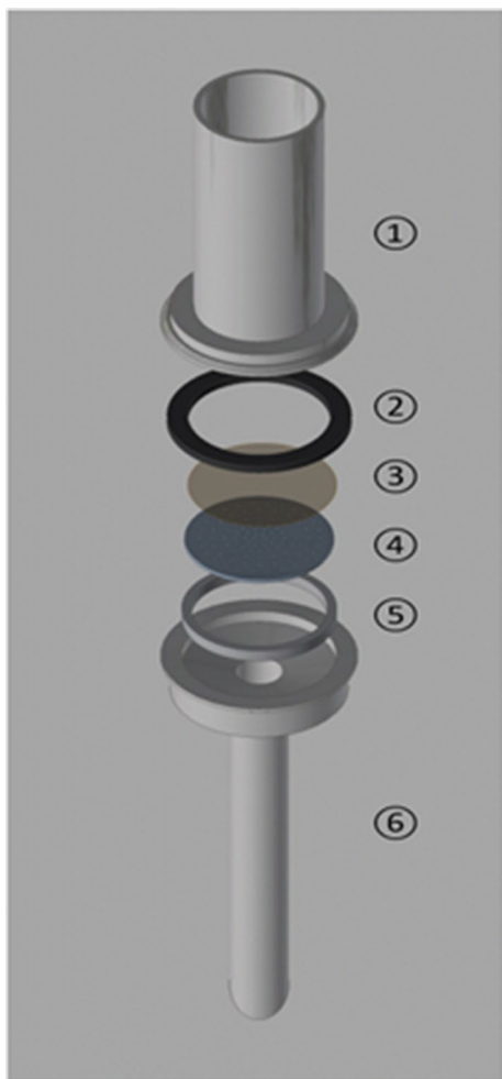
Fig. 3 Construction drawing of the filtration attachment (CAD image file); ① The upper part is composed of a stainless steel hollow cylinder (DN25) and a clamp weld-on socket ② The sealing ring provides the necessary contact pressure of the membrane filter ③ The membrane filter is inserted between the sealing ring and filter frit ④ The filter frit serves as a carrier surface for the membrane filter and defines the flow volume ⑤ The carrier ring serves as a support and fixation of the filter frit ⑥ The lower part is composed of a bevelled stainless steel hollow cylinder (DN10) and a clamp welding socket
