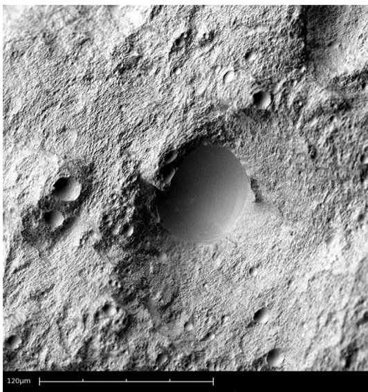
Fig. 5 SEM image of the fracture surface of a 45° polar angle specimen
