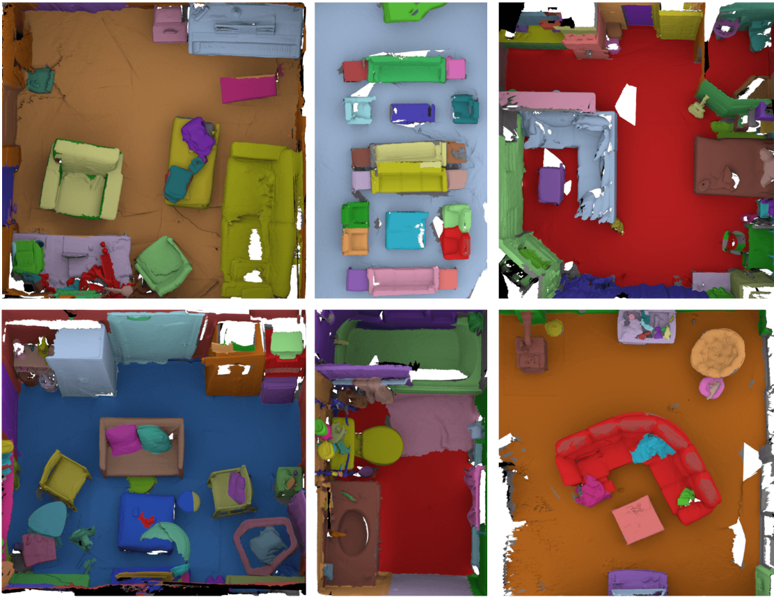
Figure 2.9: Rich annotations of the ScanNet scenes [13]. ScanNet provides instance-level semantic segmentations. Different colors represent different instances.
