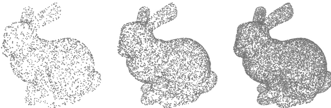
Figure 2.2: Point Cloud of the Stanford Bunny. A point cloud is a discrete set of points representing 3D geometry. Point clouds with different point coordinates and densities can still represent the same 3D shape.
