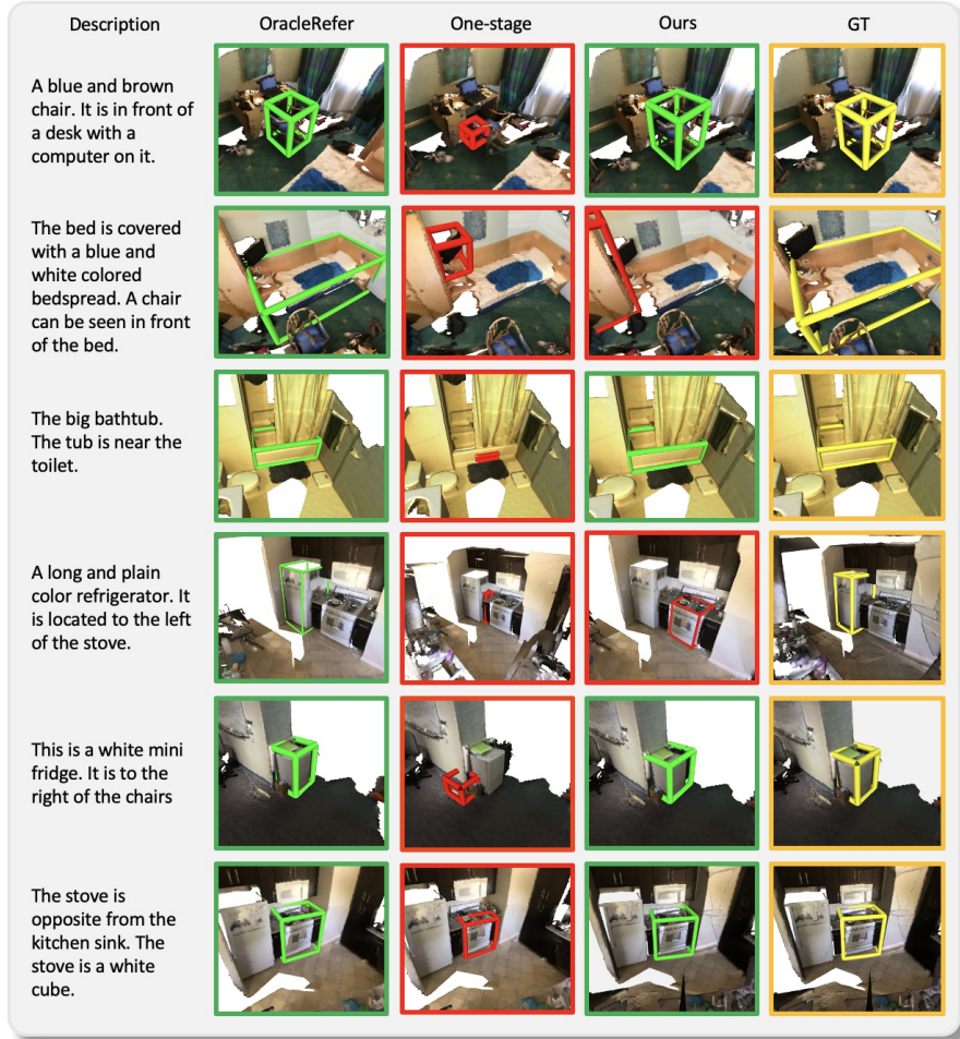
Fig. 17: Additional qualitative analysis in the “unique” scenarios where there is only one object from a certain category. Our method is capable of localizing the target object in a 3D indoor scene with the help of the free-form description.
