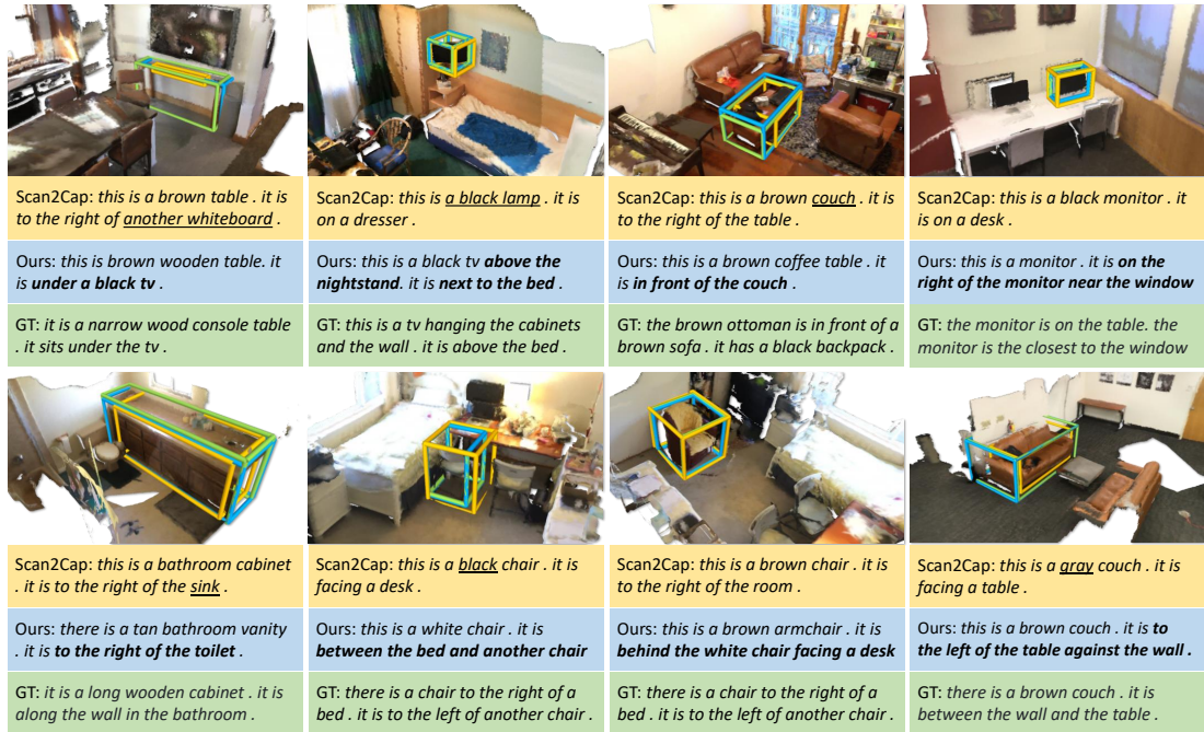
Figure 5.4: Qualitative results in 3D dense captioning task from Scan2Cap [15] and our method. We underline the inaccurate words and mark the spatially discriminative phrases in bold. Our method qualitatively outperforms Scan2Cap in producing better object bounding boxes and more discriminative descriptions.
