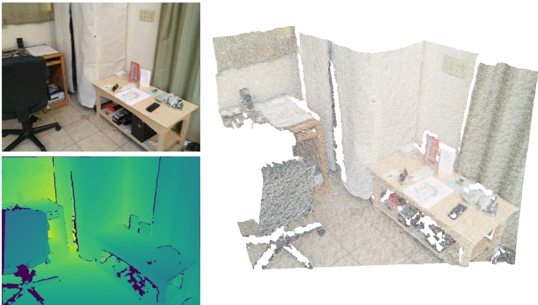
Figure 2.3: Point Cloud From RGB-D camera. We show an RGB frame (top left) and a depth map (bottom left) from the ScanNet [13]. A point cloud (right) can be generated by back-projecting the RGB values from pixel space to 3D space using the depth map.
