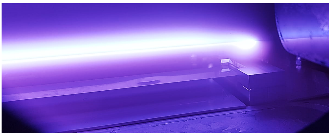
Figure 3.24: Coating process of a foil in the full-size device.
