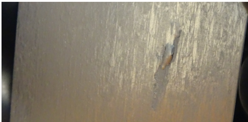
Figure 4.56: Surface defect on a coated LANL foil, where a flake of U-Mo is about to peel off.
