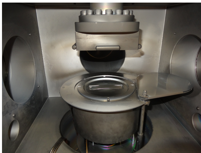
Figure 3.2: Vacuum chamber with removed front door showing the sputtering source and the substrate holder.
