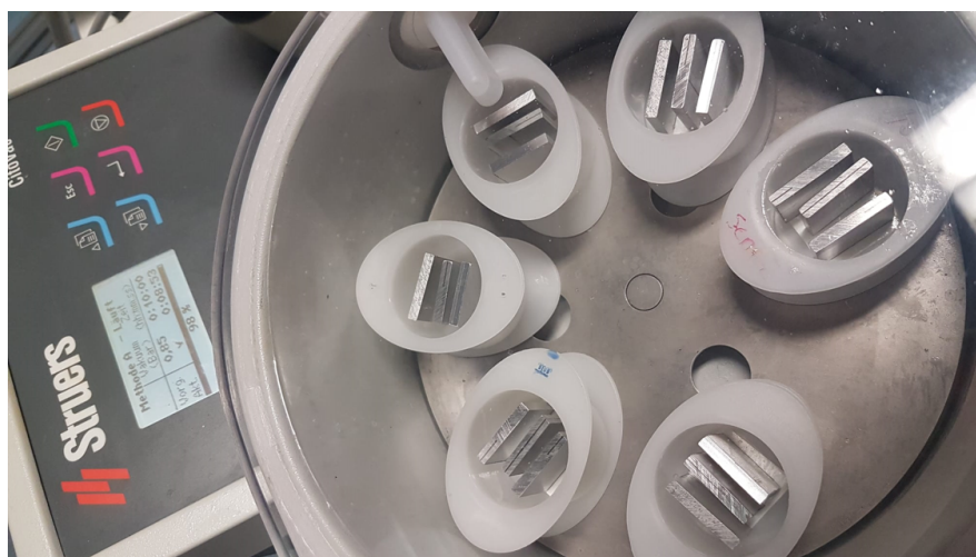
Figure 3.28: Mounting cups with sample pieces inside the vacuum impregnation unit ready to be filled with epoxy.
