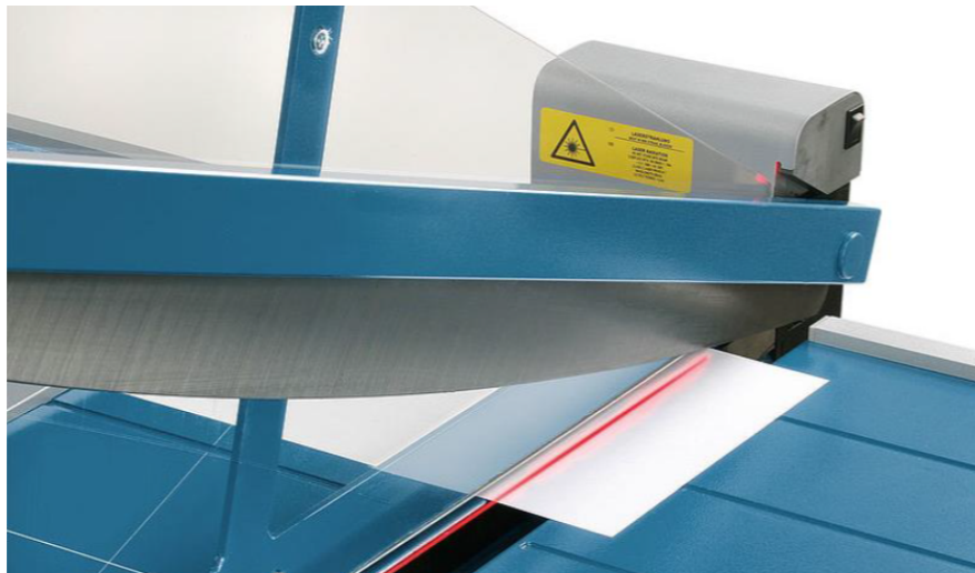
Figure 3.19: Cutting of a foil with the workshop guillotine. The red laser indicates the cutting line.
