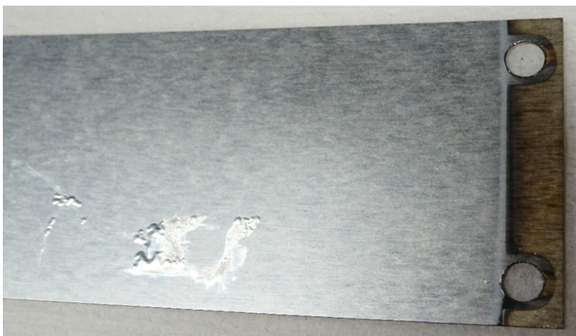
Figure 4.49: Coating defect caused by a short circuit during plasma cleaning.
