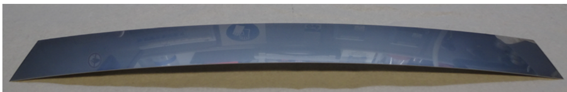
Figure 3.11: Bent half-size (380 mm length) stainless steel substrate foil after coating of one side.
