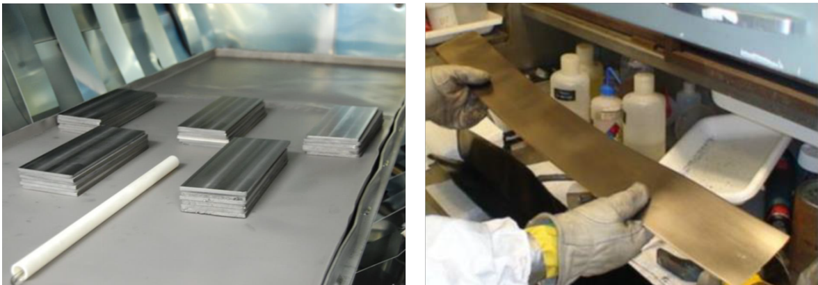
Figure 1.6: Exemplary images from the foils fabrication process. As-cast ingots prepared for homogenization (left) and a master foils after de-canning (right). From [42].
