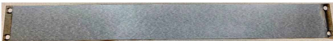
Figure 4.39: Coated half-size U-Mo foil before removal of the drilled and uncoated end pieces.
