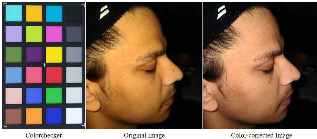
Figure 5.12: We found that the polarization filters introduce a color shift depending on the polarization direction. To this end, we perform a color calibration with a Macbeth colorchecker board which we capture in both scenarios (cross-, and parallel-polarized). We use an affine color correction to match both captures, and apply this transformation to recordings of all subjects.
