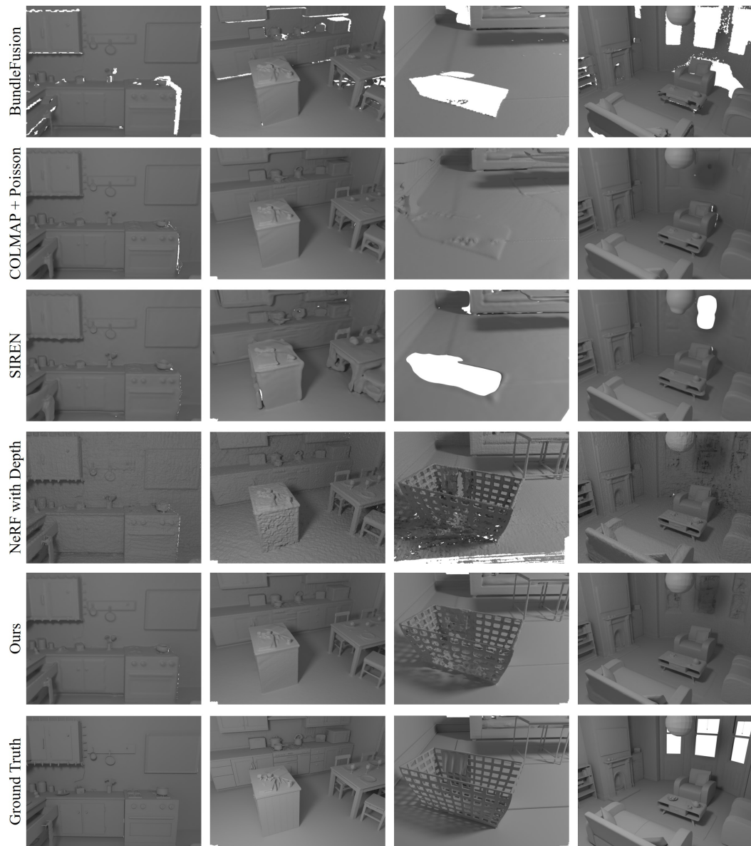
Figure 4.15: We show a qualitative comparison of synthetic scene reconstructions obtained using our method and several baseline methods. The BundleFusion reconstruction is incomplete in some regions, screened Poisson and SIREN attempt to fit noise in the depth data, while the NeRF reconstruction suffers from noise in the density field. Our method manages to fill in gaps in geometry, while maintaining the smoothness of classic fusion approaches.
