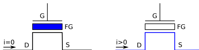
Figure 6.1: Binary 0 (charged cell) on the left and reading of a NOR flash cell, with a binary 1 (uncharged cell) on the right.
