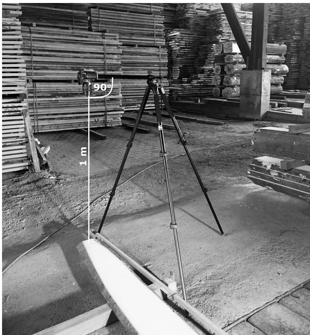
Fig. 1 Camera arrangement for the image acquisition at the Fehrensen GmbH showing the vertical distance to the board surface of 1 m and the angle to the board surface of 90° (created using INK-SCAPE version 0.92 and Adobe Photoshop CS3 Extended version 10.0; source Höwler et al. 2019)
