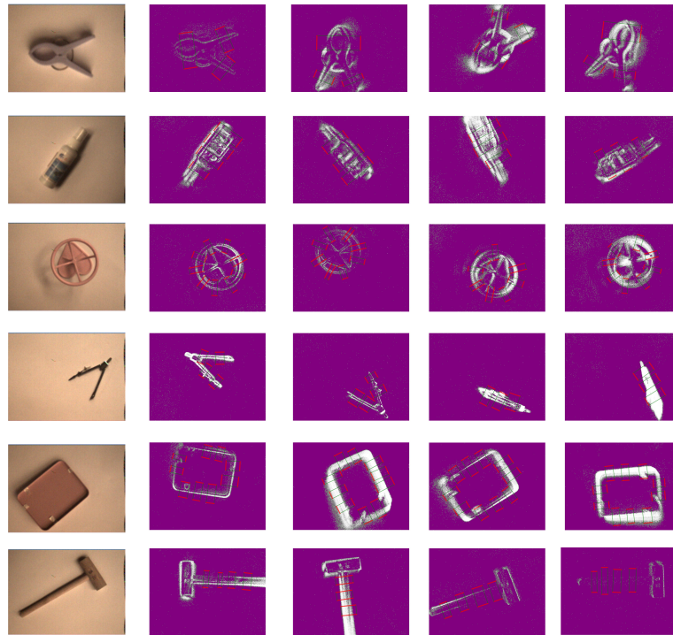
Figure 5.20: Grasp annotations: six grasping objects with different poses and views are selected for display. The first column contains RGB images, and the remaining columns contain labeled "grasping object" event data in various poses. Adapted from Fig. 6 in [Cao+22b] ©IEEE.
