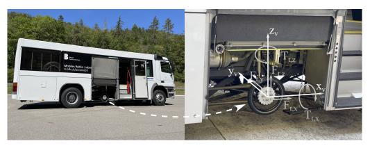
**Figure 1.** MoReLab truck and measurement chamber with mounted bicycle tire and corresponding coordinate system.
