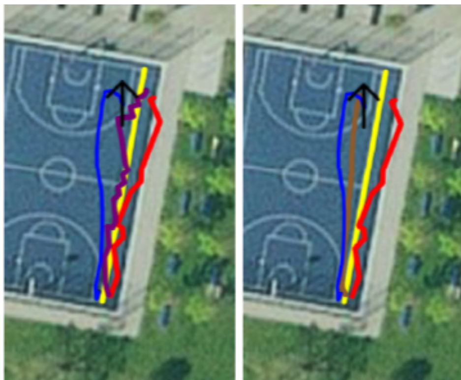
Figure 15. Jittering signal of KF Vel CT (purple) and smooth signal of KF CT (brown).
