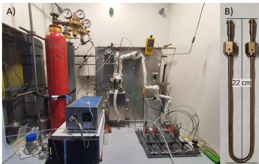
Figure 39: A) Picture of the test unit and B) picture of the U-shaped reactor.
