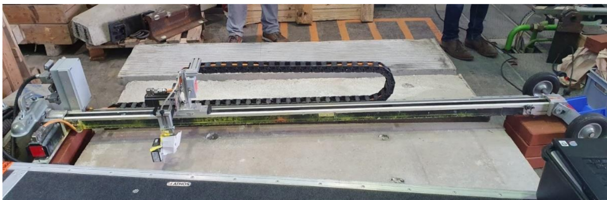
Figure 3. Laser profilometer for surface texture measurement.
