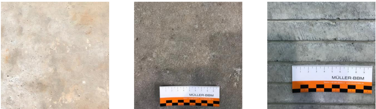
Figure 2. Detailed surface images of SHCC (left), modified SHCC-Cor (center), and SHCC-Cor-Gro (right).
