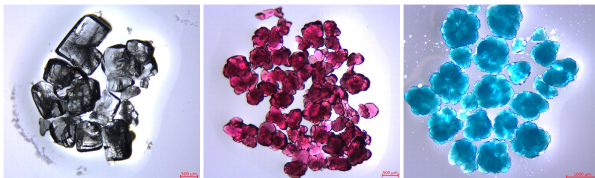
Fig. S9 Batch photographs of crystalline material [(C_3H_7)_3(CH_3)N]M(C_2N_3)_3 as synthesised in sample vials, with M being Mn^{2+} (left), Co^{2+} (middle) and Ni^{2+} (right). Crystallite sizes vary from 100 – 1000 \mu\text{m} .
