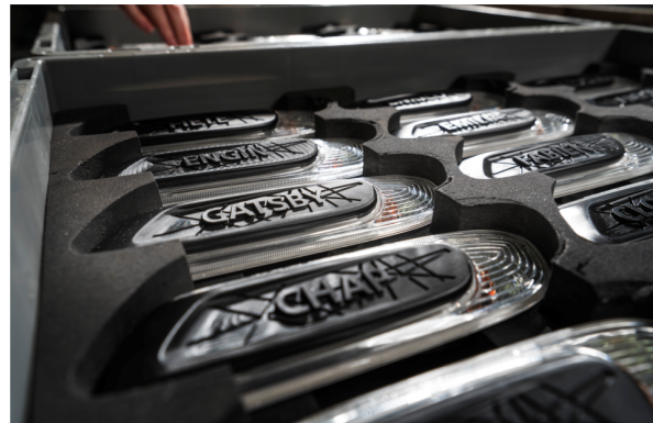
(d) Personalized MINI turn signal housings printed with RPU 70 [44]. © BMW AG.
