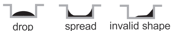
Fig. 4. Spread, drop and invalid liquid sample shape applied in open DSC crucible.
