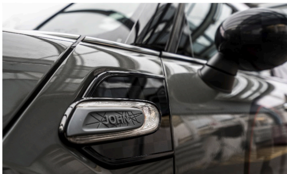
Fig. 2. Personalized MINI turn signal housing also known as side scuttle. Source: BMW press club [5].
