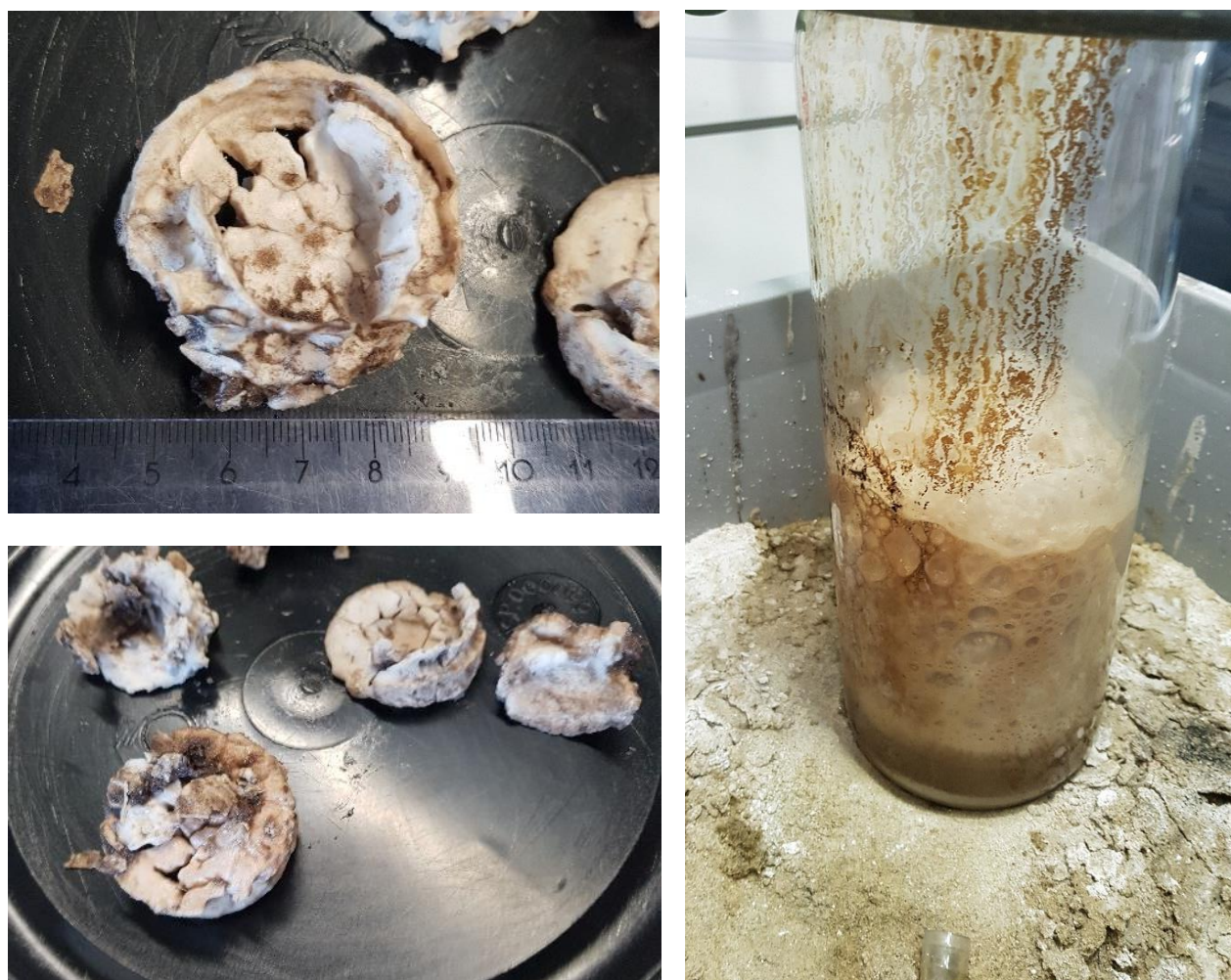
Figure 39: Two photos on the left show solid residues of the decomposition reaction floating on top of the reaction medium at the end of the decomposition. These residues consist mainly of undecomposed peroxides. On the right side, one can see the strong foam formation during an ongoing decomposition reaction, which leads to inhomogeneous mixing.
