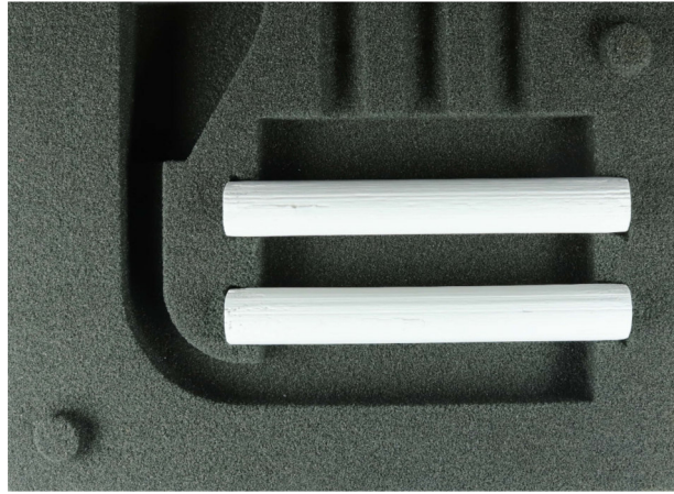
Figure 6.17: Insertion of two ceramic casting cores into a 3D printed sand mould.
