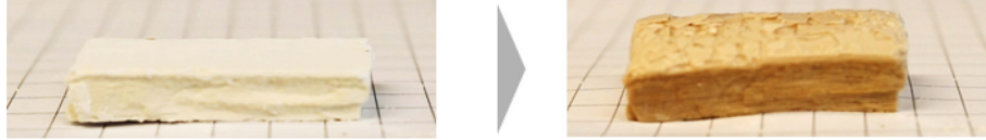
Figure 6.7: Demonstration of the expansion of a powder compact in the z-direction and its colouration followed by the saturation of the pores with water.
