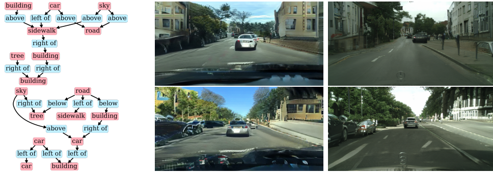
Figure 7.13: Traffic scene images generated from the same synthetic scene graph using appearances BDD and Cityscapes. © 2021 IEEE
