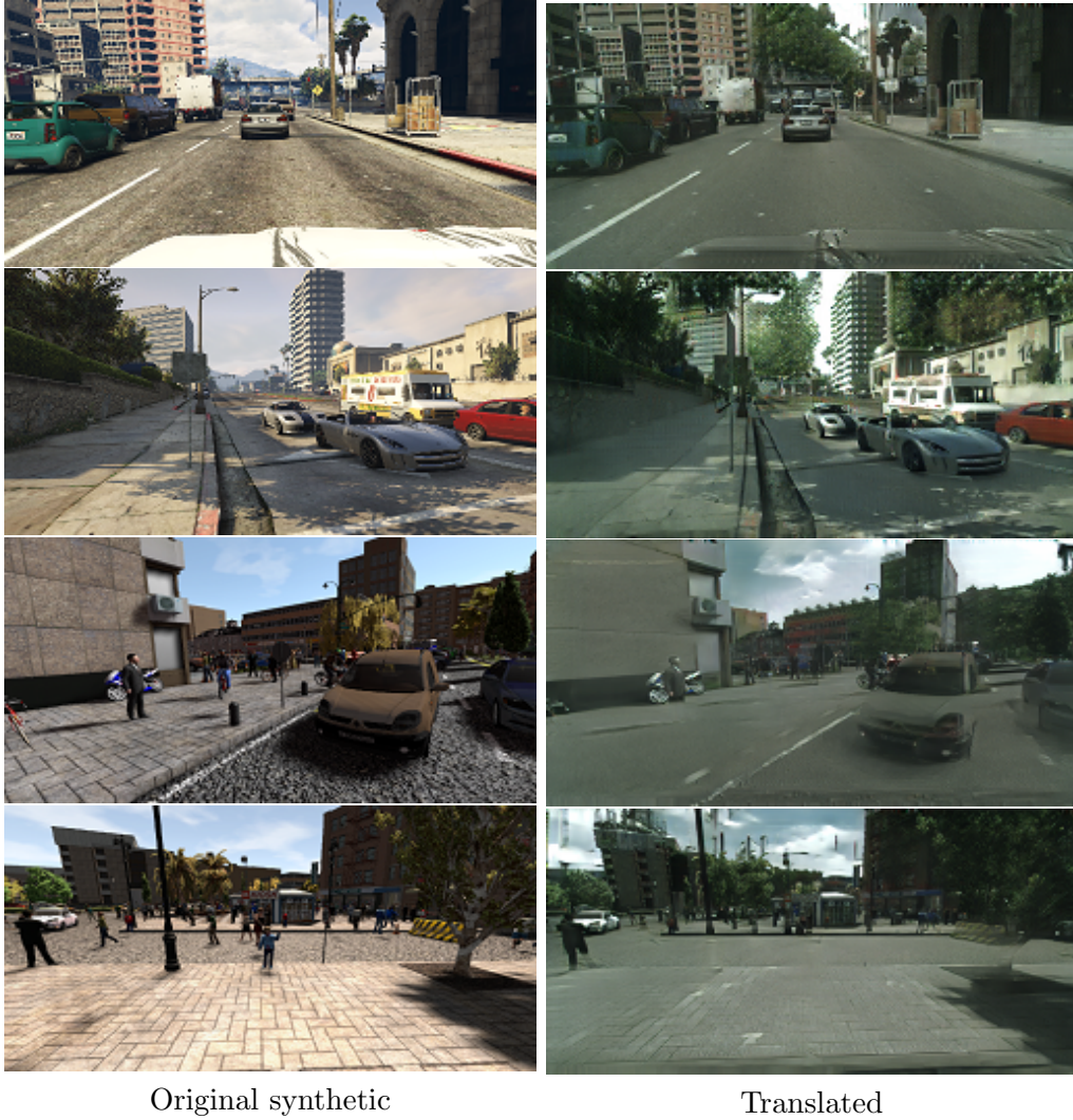
Figure 5.5: Semantically inconsistent sim-to-real adaptation performed by the adversarial network by translating Playing for Data and SYNTHIA images to the Cityscapes domain. © 2020 IEEE
